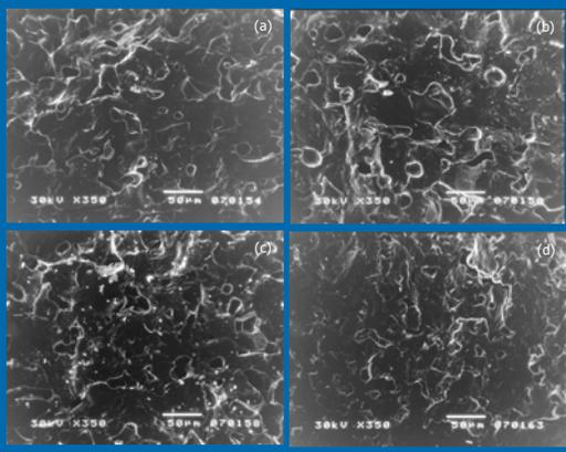
Microstructures of BaTiO<sub>3</sub> ceramics prepared from BT powders with average particle size of: (a) 1.400 μm; (b) 1.300 μm; (c) 410 nm and (d) 64 nm.
