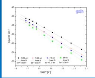
Arrhenius plot of grain and grain boundary conductivity data of BT samples sintered at 1370 °C in air
