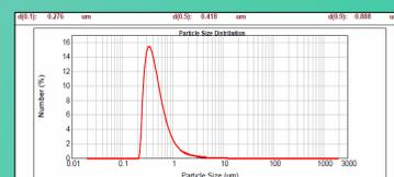
Figure 4 Particle size distribution of  $\text{LiFePO}_4/\text{C}$  powder
