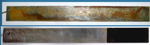
Figure 8. Comparison of the images of bare mild steel and mild steel with partial PANI-benzoate coatings after a ten-hour exposure to 3% NaCl at the corrosion potential.
