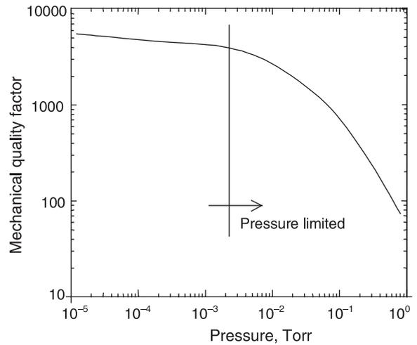
Fig. 7. Dependence on the mechanical  $Q$  factor on pressure for a silicon nitride cantilever [25].
