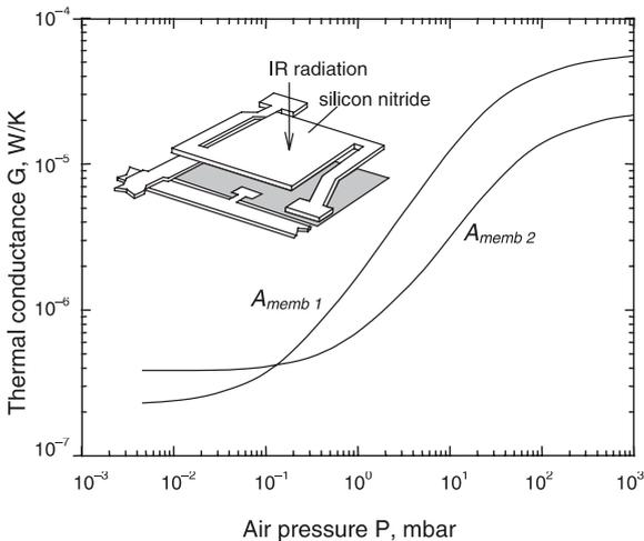
Fig. 4. Dependence of the thermal conductance on gas pressure for two membranes,  $A_{\text{memb}1} = 100 \times 100 \mu\text{m}^2$ ,  $A_{\text{memb}2} = 50 \times 50 \mu\text{m}^2$ . Detector structure is shown in the inset.
