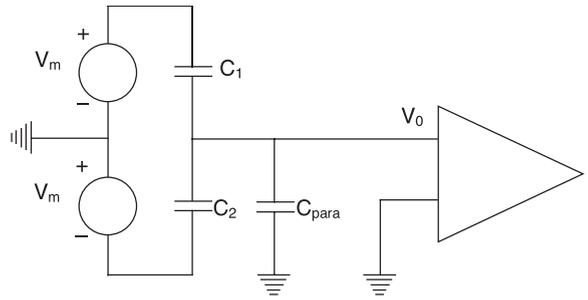
Fig. 6. Accelerometer sensing interface.
