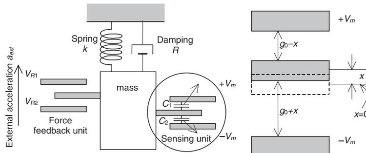
Fig. 5. Schematic representation of a capacitive accelerometer.
