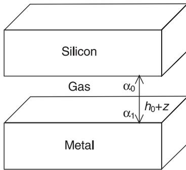
Fig. 2. Schematic of the air gap between the silicon (membrane) and the fixed metallized electrode. The air gap height  $h_0$  is much smaller than the other dimensions.  $z$  is a small variation in the plate separation,  $\alpha_0$  and  $\alpha_1$  are the accommodation coefficients.
