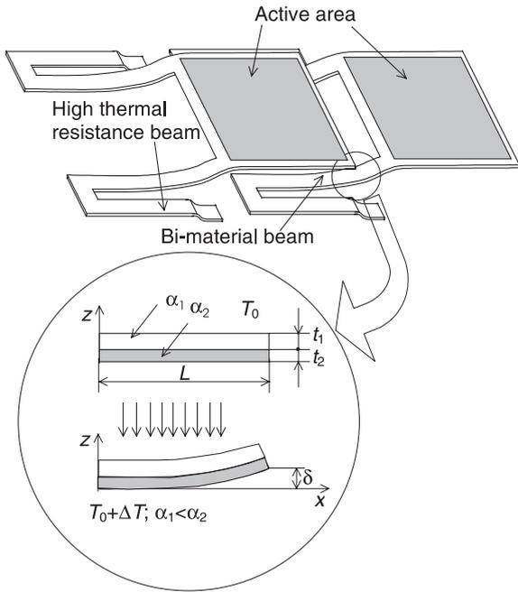
Fig. 8. The IR detector based on the bimaterial concept.
