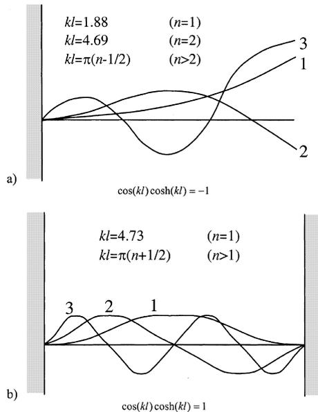
Fig. 1. Fundamental modes for (a) the cantilever and (b) the clamped-clamped beam.
