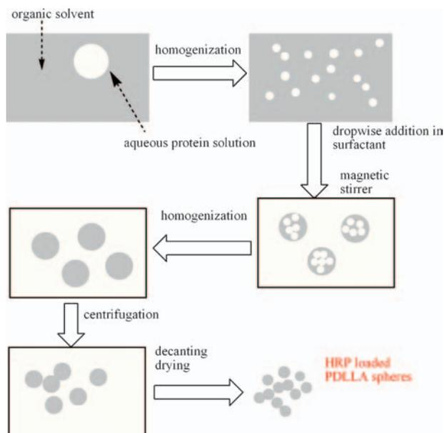
**Fig. 1.** Schematic diagram of manufacturing process for HRP-loaded PDLLA spheres.
