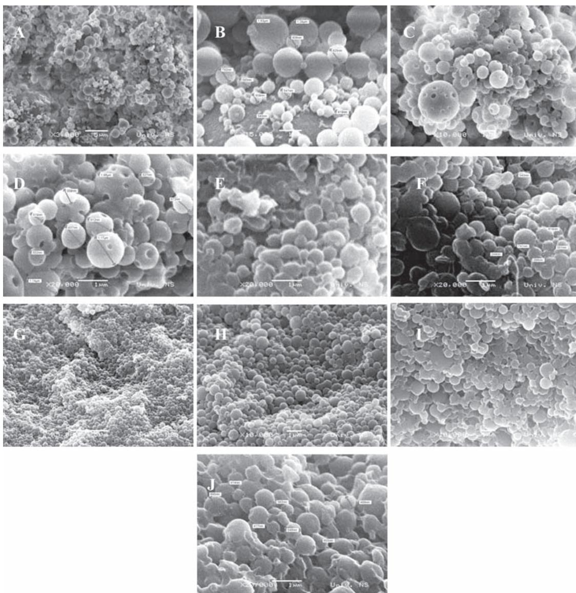
**Fig. 4.** SEM images of HRP-loaded PDLLA spheres prepared by precipitation method. The size of the bar is shown on the images. Images A and B—the first batch, images C and D—the second batch, images E and F—the third batch, images G and H—the fourth batch, images I and J—the fifth batch. All batches are listed in Table I.
