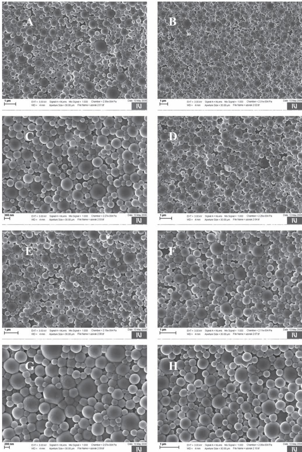
Fig. 5. FESEM images of HRP-loaded PDLLA spheres from the fourth batch (Table I) prepared by precipitation method.
